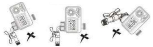
• **Tips:** If the connection between the timer and the faucet or hose is not tight or leaking, wrap more Teflon Tape(thread seal tape) to make them tight.
