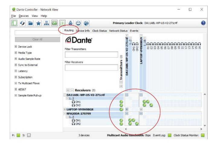
It is also possible to change the settings of the DA11ABL-WP-US-V2 under the "Device Info" screen in the Dante Controller software. To do so, select the "Device Config" menu. Here we can adjust the sample rate and the encoding bit rate of the DA11ABL-WP-US-V2. Please note that Dante products can only transmit or receive audio from other Dante products that are set up with the same sample rate. A mismatch in sample rate may stop audio from transmitting.
