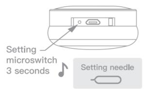
**WARNING:** Please do NOT push the needle too hard as this can cause damage to the setting microswitch. A click should be felt as the needle makes contact with the microswitch, when operated correctly.
