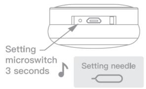
**WARNING**: Please do NOT push the needle too hard as this can cause damage to the setting microswitch. A click should be felt as the needle makes contact with the microswitch, when operated correctly.
