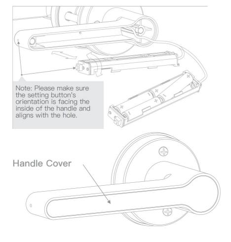
Pull out the battery cassette and change the batteries. Put the battery cassette back into its original position (see diagram) and ensure the cable is still connected. Put the handle cover B-1 back on.
