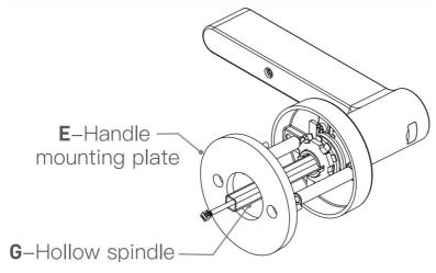
Push the mounting plate (E) over the spindle and connection bosses until it's flush with the handle.
