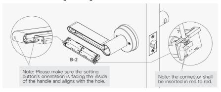
9. Test the handle. Push the internal handle down, it should operate the latch fully. then touch the fingerprint sensor on the external handle, it should light up GREEN and you should hear the mechanism turn. push the handle down and it should operate the latch.
