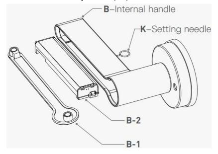
7. Take the second mounting plate (E) and place it over the spindle. holding the internal handle (B), feed the wire and spindle through the spindle hole in the handle You will be able to see the cable coming through from the back of the handle. use the screws provided (I) and fix the internal handle to the external handle through the holes Screw the exposed fixing first so that you can push the handle down to fit the second screw.
