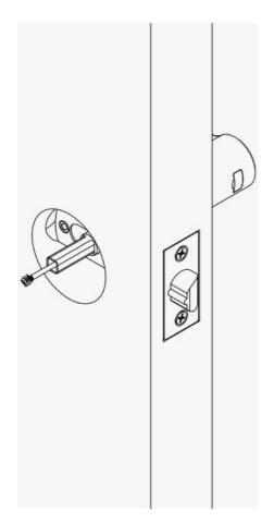
6. Place the internal handle (B) and the setting needle (K). At the back of the handle grip, there is a small hole. Push the setting tool into this hole and press hard until the magnetic handle cover (B-1) pops off. remove the cover and also the battery cassette (B-2).
