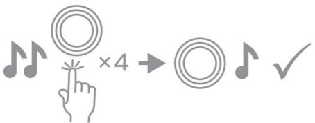
**Note:** A total of 3 ADMIN and 47 USER fingerprints can be registered. Once all fingerprints are registered, 1 triple beep will sound and the LED will turn off indicating that the USER capacity is full.
