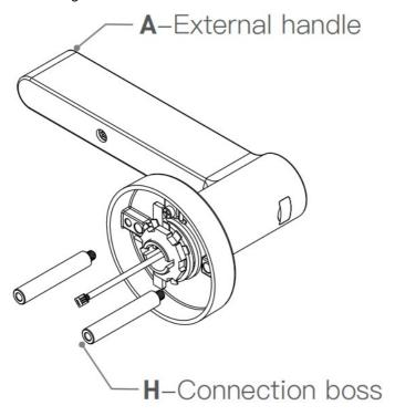
4. Take the spindle (G) and feed the wire through the hollow opening, then push the spindle into the handle.
