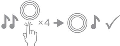
**Note:** If you want to continue setting the second and third ADMIN fingerprints straight after the first one, repeat step 2c when the LED remains BLUE. If you want to set up the second and thrid ADMIN fingerprints at a different time, wait till the LED turns off and then follow step 2d below.
