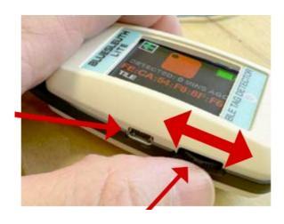
**POWER** – Press toggle button to turn unit ON. Hold in toggle button for a few seconds to turn unit back OFF
