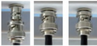
Inserting Twisting Attached Attaching the BlueLab pH Probe to the Meter
