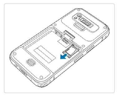
2. Insert a nano SIM cards into the slots. Make sure that the gold contacts on the cards are facing down.
