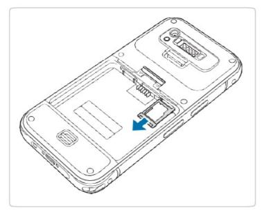
2. Insert a micro SD cards into the slots. Make sure that the gold contacts on the cards are facing down.
