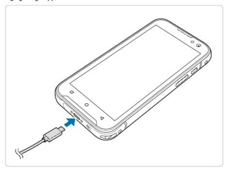
2. Connect the USB cable with power adapter and then plug the charger into a power outlet.
