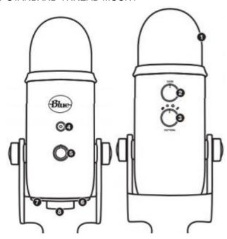
If you would like to mount your Yeti to a standard microphone studio mount, remove Yeti from the included desk stand and thread in a standard threaded mount. For broadcast applications, we recommend the Compass desktop boom arm. To isolate Yeti from noise, shock, and ambient vibration, add the Radius III shockmount.
