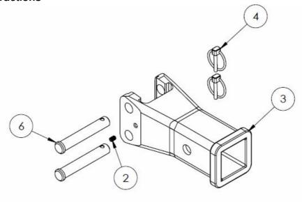
1. Install the adjustable receiver onto the receiver shank, using the 5/8" x 3-11/16" pins with 3/16" x 1-1/4" lynch pins above primary receiver. Ensure that the add-on receiver and products use with the addon receiver do not interfere with primary receiver or flat towing products.
