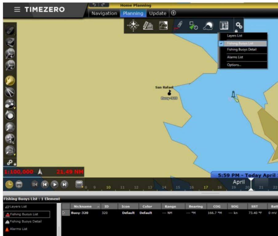
Double click the arrow on the left of a row in the Fishing Buoys List to select that buoy in the Fishing Buoys Detail panel. Here you can see the position history for the buoy. Double click an entry in this table to select it on the map.
