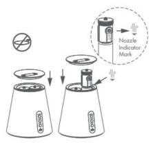
4. Insert the diffusion head & bottle into your chosen pod, ensuring diffusion head air inlet is lined up with the symbol and grooves. Place the metal cover back on top.
