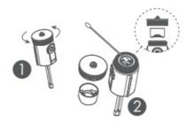
3. Rotate the nozzle cap anti-clockwise and take out the inner cap. Dip a cotton swab in the rubbing alcohol and use it to gently wipe inside the nozzle.
