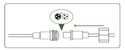
2. Step: Firmly screw the wire nut.
