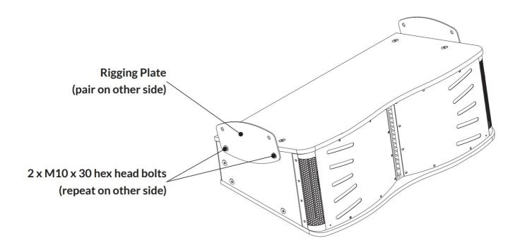
**Step 3.** Place the Rigging Grid on the top of the loudspeaker and align its attachment holes with the corresponding holes in the left and right Rigging Plates. Secure the Rigging Grid to the Rigging Plates using the supplied M10 hex head bolts with the supplied lock washers and nuts.
