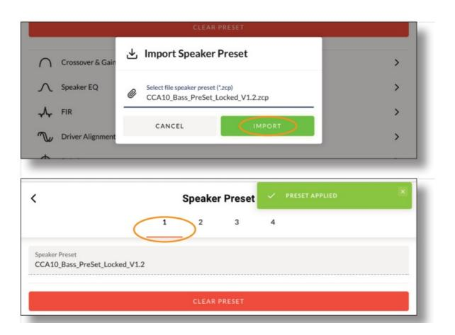
**Step 7.** With the appropriate speaker preset file (CCA10\_Bass\_ PreSet\_Locked\_V1.2.zcp ) applied to amplifier Output 1, repeat Step 2 to Step 6 for the three remaining amplifier outputs. The appropriate speaker preset files
