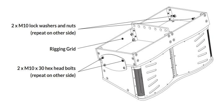
**Note:** A steel Rigging Grid is available to order for installations where specific structural and regulatory demands require it.
