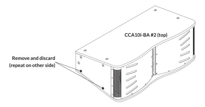
**Step 3.** Align the top CCA10i-BA loudspeaker over the bottom CCA10i-BA loudspeaker and install the provided Rigging Plates plates between the two enclosures on the left and right sides. Secure the Rigging Plates using the supplied M10 hex head bolts.
