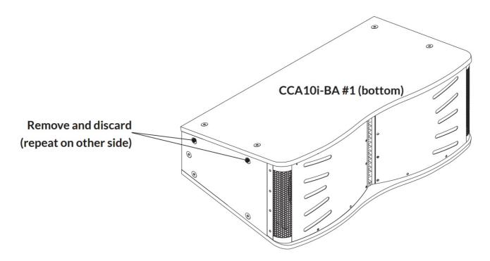
**Step 2.** On the top CCA10i-BA loudspeaker remove the two lower-most countersunk M10 bolts on the left and right sides. The bolts can be discarded.
