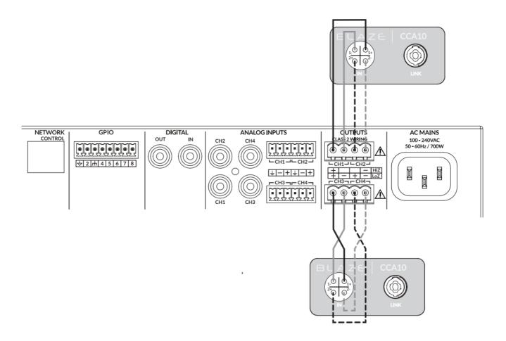
CCA10i-BA loudspeaker and PowerZone 3004 amplifier connections are illustrated in the diagram.
