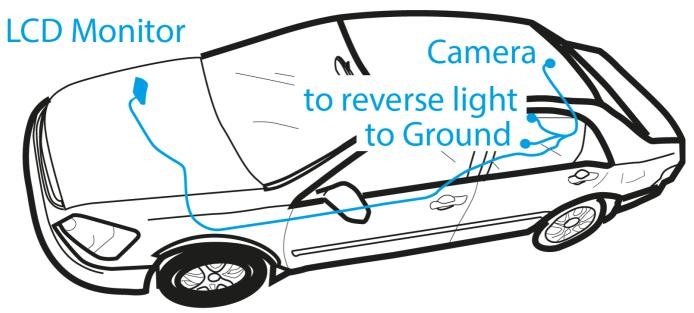
The wiring diagram applies to most (but not all) camera models, and when making the connections, please also refer to the labels or marks on the wires.
