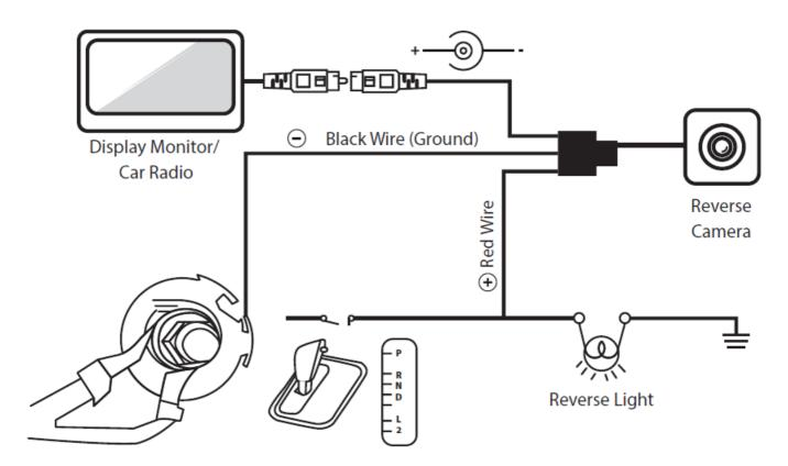
Ground the wire through the exterior body of the vehicle and keep connection intact.
