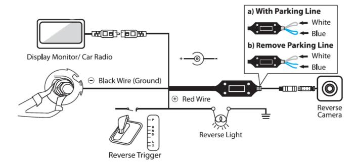
• Ground the wire through the exterior body of the vehicle and keep the connection intact.
