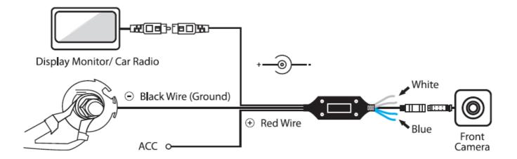
• Ground the wire through the exterior body of the vehicle and keep the connection intact.
