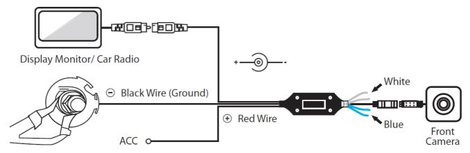
Ground the wire through the exterior body of the vehicle and keep connection intact.
