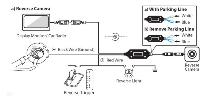
Ground the wire through the exterior body of the vehicle and keep connection intact.
