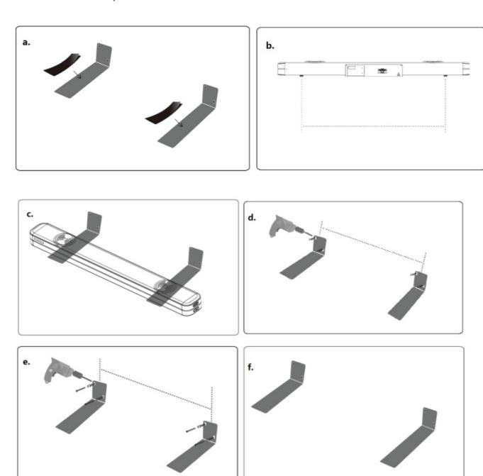
**Warning:** If you are not confident to wall-mount the soundbar correctly and securely, please seek the assistance of an experienced and skilled person of professional. Install the speaker on a vertical, reinforced area of wall. For plastic walls, it is recommended to screw into wall studs for greater security. For optimal performance, allow at least 25mm/1" distance between the soundbar and TV.
