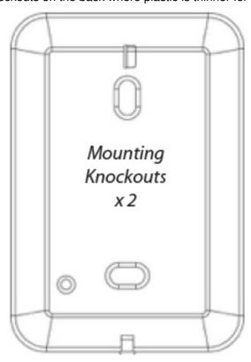
1. Use the two knockouts on the back to mark the position on the wall at chest height. Open the back cover.
