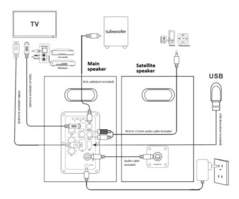
Speaker connect with outsourcing devices like TV, TV set-top, DVD, Blue-ray DVD player, MP3 player etc. The speaker has included digital (optical & HDMI(ARC)) and analogue (Line in) inputs for different source. You can reference below instruction and above drawing for the connection depends on what input jack has on your
