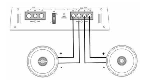
Blaupunkt Speakers wired in parallel to a single channel Total Impedance: 2 ohms x channel
