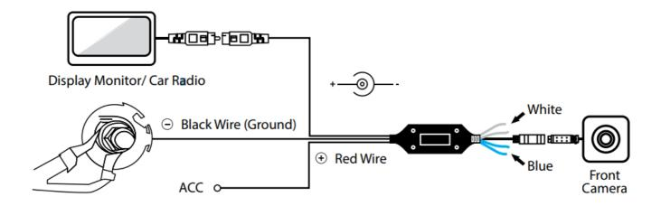
Ground the wire through the exterior body of the vehicle and keep the connection intact.
