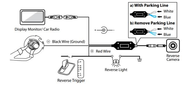
Ground the wire through the exterior body of the vehicle and keep the connection intact.
