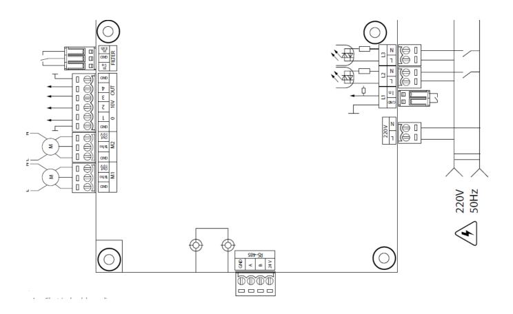
Controller power supply: 100-250 V, 50 (60) Hz, maximum power consumption – 30 W.
