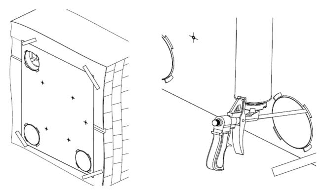
5. To install an additional extract spigot, remove the plug on the rear part of the unit. Undo the screws, remove the plug and fix a spigot on its place using screws.
