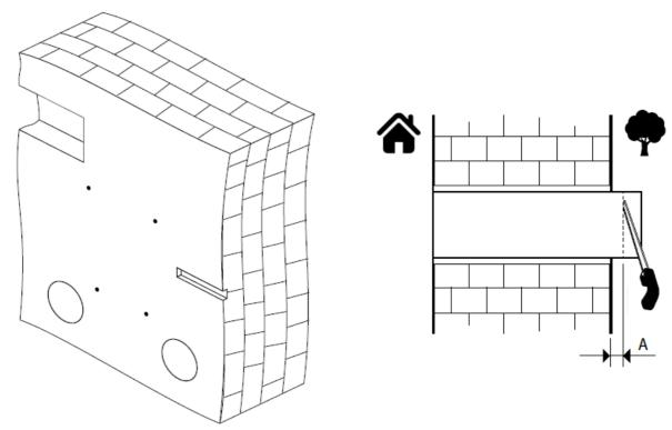
2. **Cut air ducts of the required length**. Note that the telescopic air duct end must protrude for the distance that enables installation of the outer ventilation hood. For details, refer to the installation instruction for the ventilation hood.
