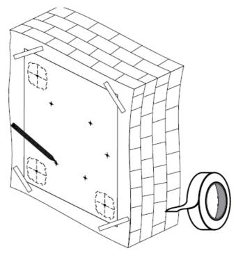
Remove the mounting template and drill two through holes Ø 120 mm for round air ducts.
