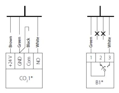
Connecting the humidity sensor or CO2 sensor to the control unit via a cable, which is attached to the bracket
