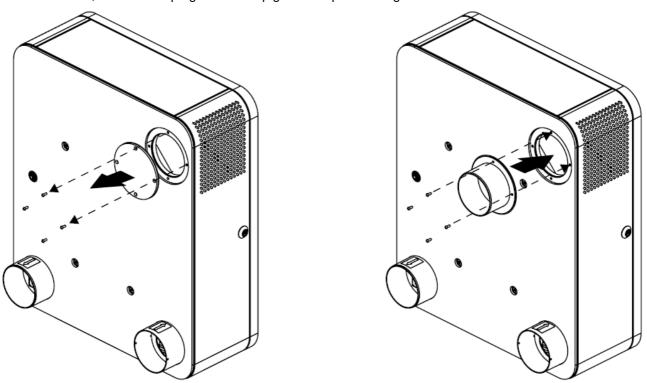
6. **Caution!** Install the condensate preheater before fixing the unit to the wall (see the Installation manual of the heater).
