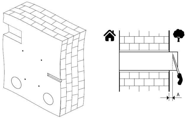
4. Fill the spaces between the air ducts and the wall with a mounting foam through the specially designed holes in the mounting template.
