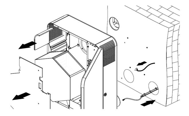
**Caution!** Remove the magnetic plug from the exhaust grille if an additional extract spigot is not installed.
