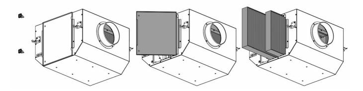
The technical maintenance of the electrostatic filter includes periodic cleaning of the surfaces from accumulated dust and dirt. Clean the electrostatic filter with a soft brush or a vacuum cleaner. Clean the filter with care. Avoid water ingress to electrical components.
