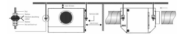
To get the best performance of the ventilation system and to minimize turbulence-induced air pressure losses, connect the straight air duct section to the spigots on both sides of the unit while installing. Minimum straight air duct length: equal to 1 air duct diameter on intake side equal to 3 air duct diameters on outlet side
