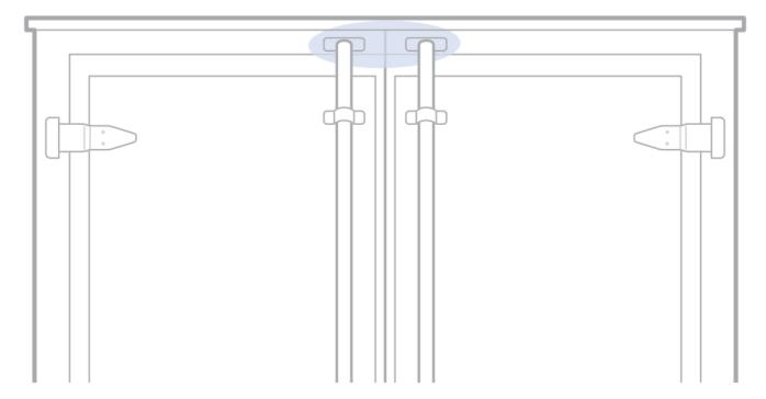
Fasten the rear camera mounting bracket using the included screws to the top of the back of the vehicle.
