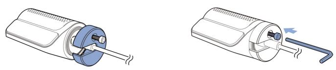
Connect the rear IR camera ('Rear' port) and main unit ("Option") using the rear camera connection cable.
