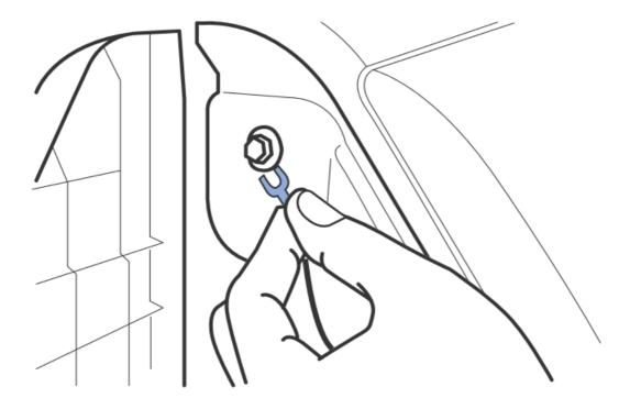
Connect the power cable to the DC in terminal of the main unit. BlackVue will power up and start recording. Video files are stored on the microSD card.
