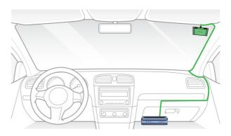
Connect the main box (USB port) and the connectivity module cable (USB).
