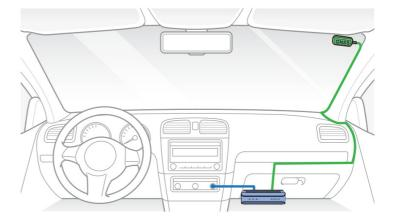
Insert the cables into the cable cover and connect them to the USB socket.
