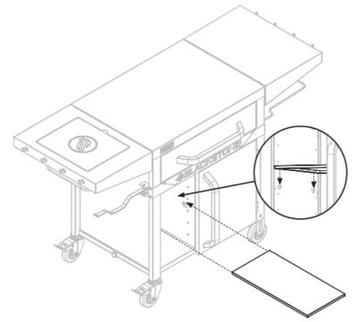
• STEP 21: Set the inner shelf onto the panel brackets.
