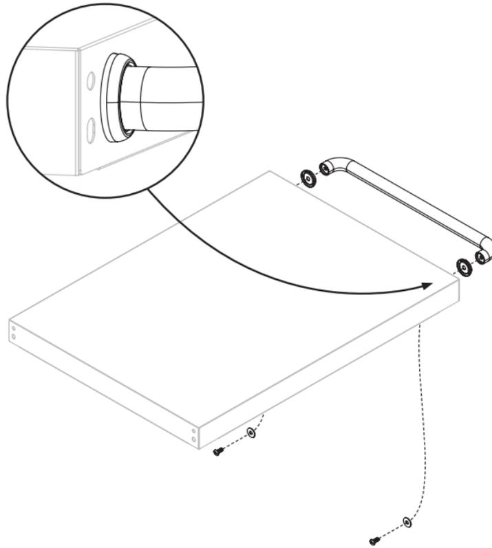
**STEP 05** Use eight (8) M6x15 bolts to attach the table top to the leg assemblies.
