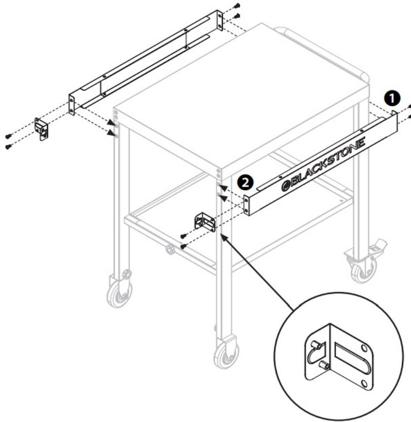
**STEP 07** Use two (2) M6x15 bolts to attach the paper towel holder to the right leg assembly.
