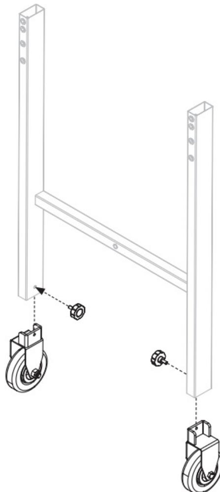
**STEP 02** Use two (2) M12 cap nuts and two (2) M12 spring washers to attach two (2) caster wheels to the bottom of the right leg assembly.
