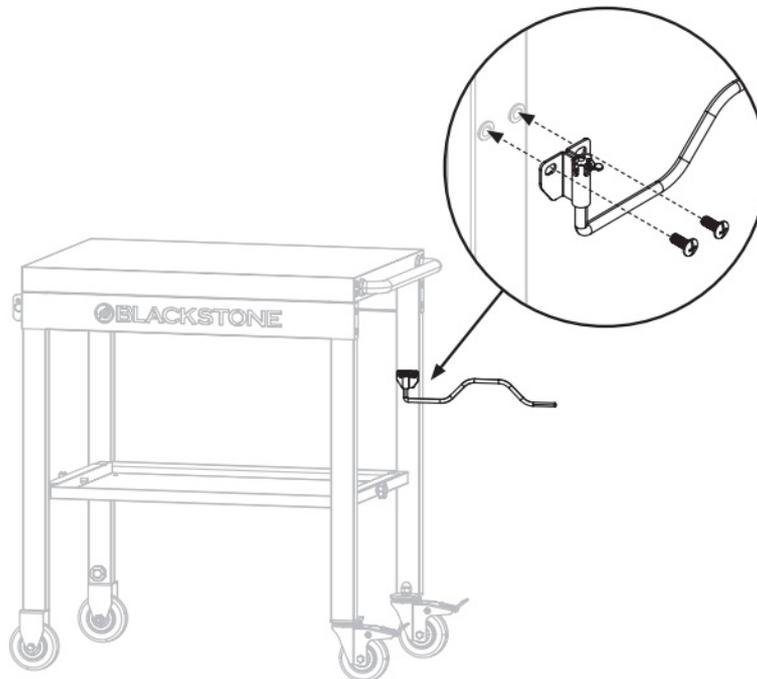
**STEP 08** Use four (4) M4x10 step bolts to attach the garbage bag holder to the garbage bag holder brackets.
