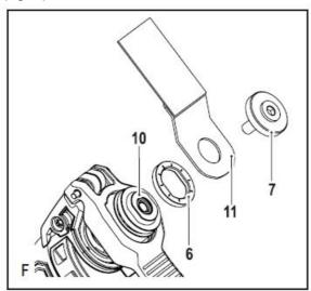
• Place the spacer (6) onto the collar (10).
