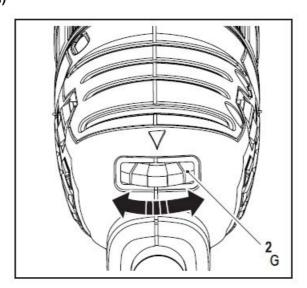
The variable speed control allows you to adapt the speed of the tool to the application.
