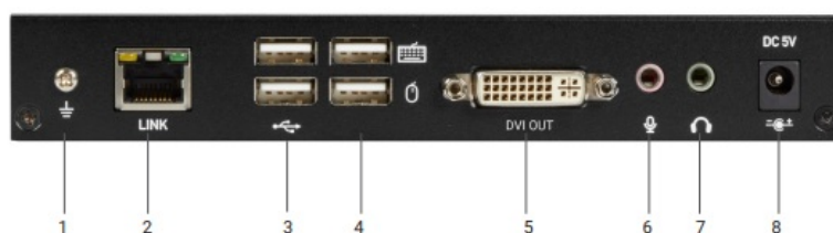
FIGURE 2-9. SINGLE-HEAD CATX RECEIVER BACK PANEL
