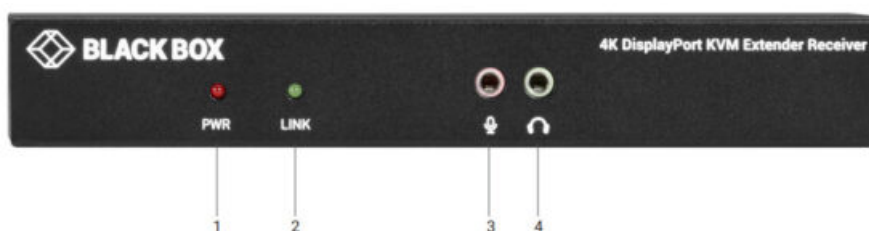
FIGURE 2-7. SINGLE-HEAD RECEIVER FRONT PANEL
