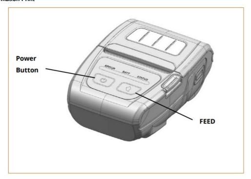
Turn the printer power off and close the printer paper cover. Then press and hold both paper feed and power button simultaneously to turn on the printer. After printing Self-Test begins, release the two buttons
