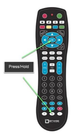
Hold the OK and B buttons simultaneously until the red status LED comes on solid (approximately 3 seconds)
