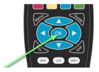
Press OK to store the new address. The red status LED will flash twice if successful. The LED will flash five times if an invalid address was entered or if the procedure times out.
