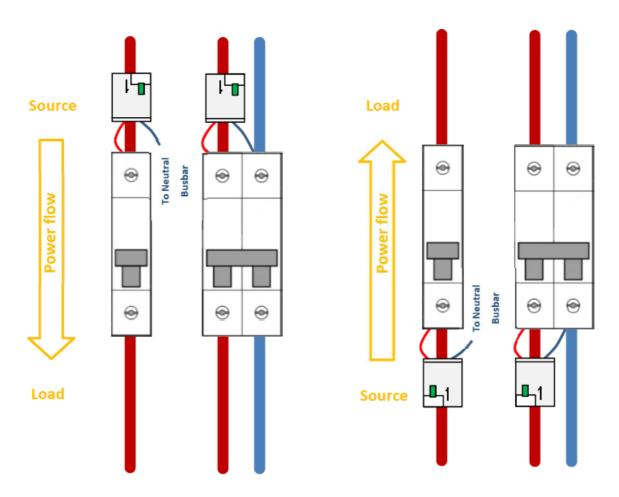
SPM01 Smart Energy Sensor / Monitor with Wireless-communication for 1P+N System
