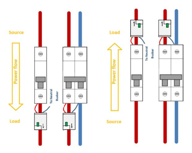
**Note:** SPM01 can be damaged, if it is installed downstream of switching devices – such as a contactor, frequency converter or motor starters.
