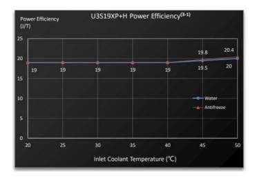
(3-1) The hashrate value, and power efficiency on wall are all typical values. The actual hashrate value fluctuates by  $\pm 3\%$ , and the actual power efficiency on wall fluctuate by  $\pm 5\%$ .
