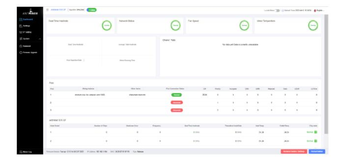
**Note**: The S19 XP server (141T) is with fixed frequency 485 MHz. Firmware will stop running when the Temp (Outlet) reaches to 75°C there will be an error message "over max temp, pcb temp (real-time temp)" shown on the bottom of the kernel log page. Meanwhile, the server temperature on the dashboard interface turns abnormal and shows "Temp is too high".
