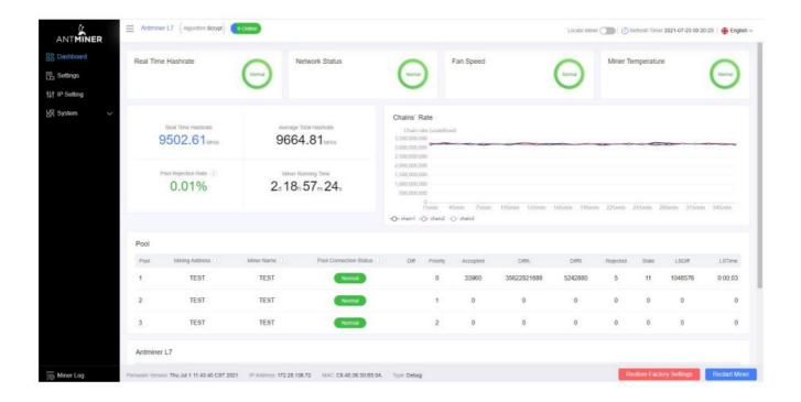
Note: The L7 server (9500T) is with fixed frequency 1850 MHz. Firmware will stop running when the Temp (Outlet) reaches to 80there will be an error message "over max temp, pub temp (real-time temp)" shown on the bottom of kernel log page. Meanwhile, the server temperature on the dashboard interface turns to abnormal and shows "Temp is too high".
