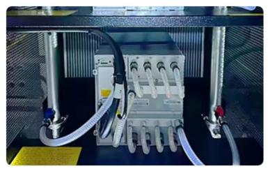
2. Connect the waste heat module to the ANTRACK's front interface.
