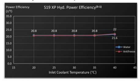
The hashrate value, and power efficiency on wall are all typical values. The actual hashrate value fluctuates by  $\pm 3\%$ , and the actual power efficiency on wall fluctuate by  $\pm 5\%$ .
