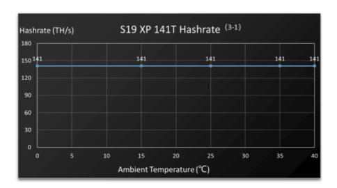
(3-1) The hashrate value, and power efficiency on wall are all typical values. The actual hashrate value fluctuates by  $\pm 3\%$ , and the actual power efficiency on wall fluctuate by  $\pm 5\%$ .
