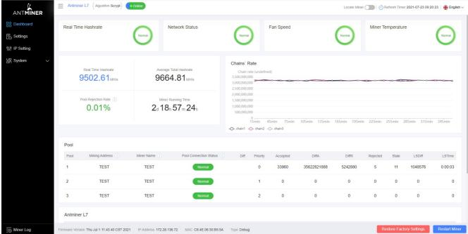
**Note:** The L7 server (9500T) is with fixed frequency 1850 MHz. Firmware will stop running when the Temp (Outlet) reaches to 80°C there will be an error message "over max temp, pcb temp (real-time temp)" shown on the bottom of kernel log page. Meanwhile, the server temperature on the dashboard interface turns to abnormal and shows "Temp is too high".
