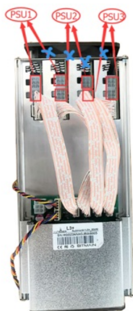
Figure 2-1. PCI-E Connectors - Correct Connection
