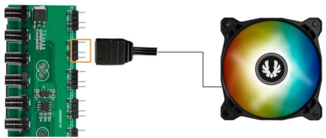
• How to connect fan header on Tracery 6+6 Controller Each connector support up to 6 fans
