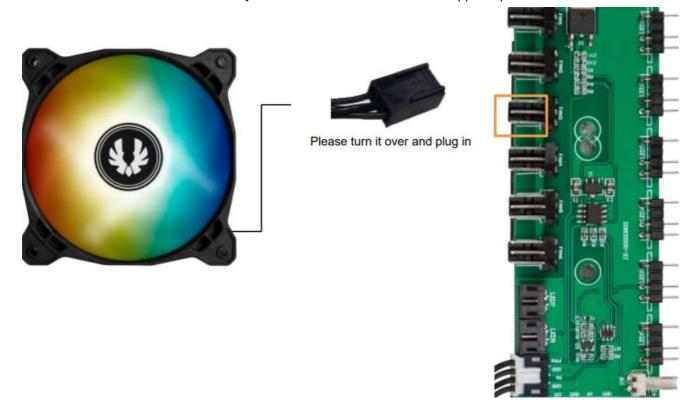
How to connect by Motherboard Addressable RGB 3pin connector
