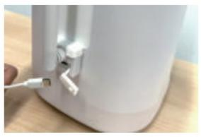
2. Thread the charging cable through the rubber plug.
