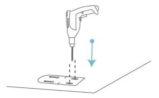
The installation steps are the same as for wall installation, but the Screw Bracket is installed at the bottom and fixed to the ground.
