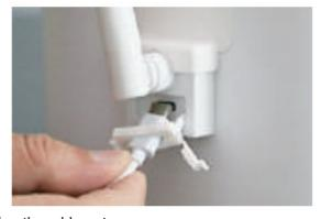
3. Insert the charging cable and firm the rubber stopper.
