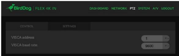
BirdDog FLEX 4K IN and FLEX 4K BACKPACK can control external PTZ cameras from the RS-232 serial port using the Sony VISCA protocol.
