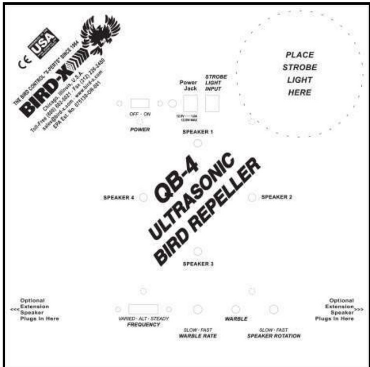
Diagram IV-c: QB-4 Control Panel
