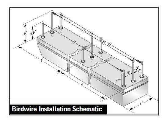
Bird-X, Inc.'s Birdwire system is used worldwide to deter pigeons and larger birds from roosting on exposed building ledges, parapets, window sills, pipes and roof peaks. The system features hard-to-see ultra violet protected, nylon-coated stainless steel wire spring-tensioned between stainless steel posts.
