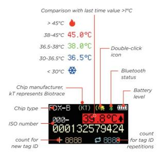
On SCAN menu to press button to start chip read- ing for 10 seconds. A transponder is detected, the reader emits a 'beep' and displays the chip infor APP for firmware upgrading/record data export- ing, etc.
