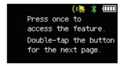
mation as the above image shows. If no transponder is detected after 10 seconds, the screen will display 'NO FOUND'. This message will be erased and restart the scanning after another press of the button.
