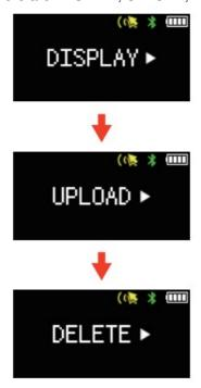
On RECORD menu, press the button to enter the sub-menu, on the sub-menu, double-click to navigate the sub-menu from DISPLAY, UPLOAD to DELETE.
