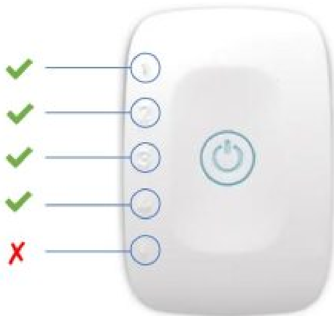
Figure 5: EDA compatible biosignalsplux channels (green checkmarks).
