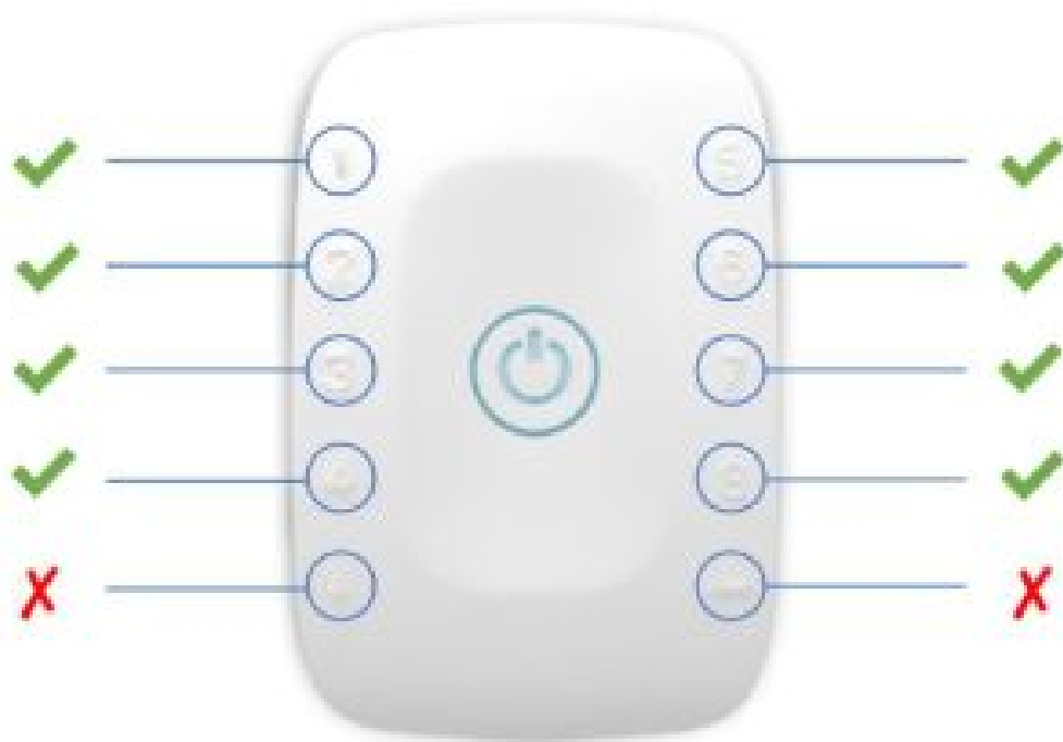
Figure 6: EDA compatible biosignalsplux channels (green checkmarks).
