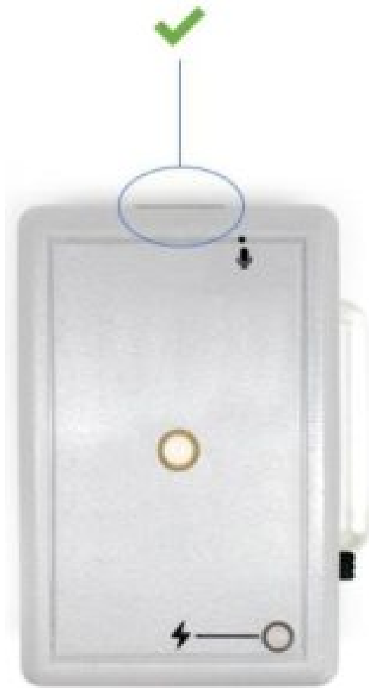
Figure 7: Connect the EDA to the analog input channel of the biosignalsplux Solo (openBAN).
