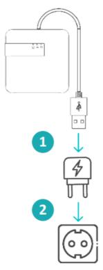
Connect the terminal cable to the charging adapter.
